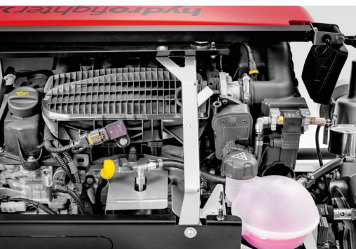
Water-cooled 3-cylinder 4-stroke gasoline engine, silent engine operation with low vibration, exhaust gas cooling system
