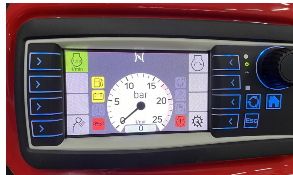
Self-illuminating color display with rotary control for speed adjustment and pump pressure control
