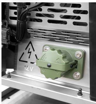
"NATO" jump start socket 12V DC and OBD II diagnostic connector
